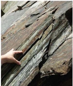
Brittle fracture cutting through solid rock in rock slope near Lake Louise
